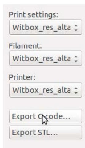
When the .gcode has finished exporting you can remove the SD card from the computer and insert it in the Witbox. From the LCD panel you can navigate to “Print from SD” and choose the file you wish to print.
