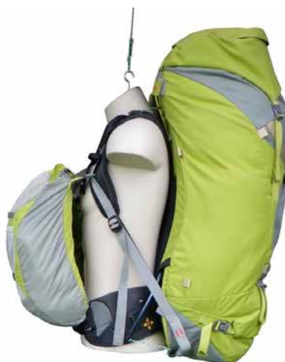
Hanging packs to show significant shift in center of gravity with front balance pockets Supplied by Aarn Tate
