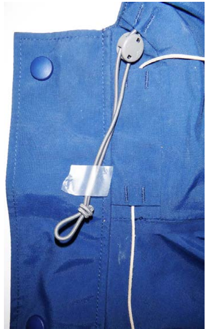
The hood gripper arrangement. The white cord shows where the hood cord was, under the flap. Note the gripper was in a very tight place, hard to grab. The gripper cord had to be taped to keep it in frame.
