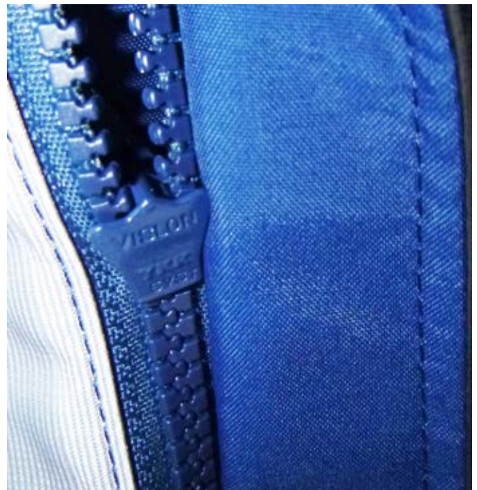
Zip catching on the inside flap before it was removed
