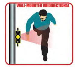
powered on, even small amounts of ferrous material passing anywhere in between the units, from ground level up to 75 inches above the ground, will trigger an alert. Poles will only trigger while someone is moving between them meaning security staff can move freely around the portal without triggering any alert.
