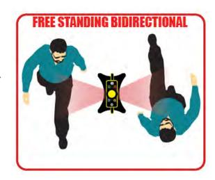
Note: If ferrous material passes by the unit at the same time that someone else moves near the portal, there is a risk of false detection. SafeHound should always be setup in an area with minimal ferromagnetic activity. This activity can include large moving ferrous objects such as wheeled office chairs, filing cabinet drawers, steel doors and even large trucks in a nearby parking lot.
