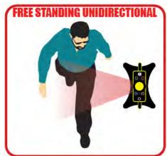
The alert LEDs on one side of the poles, the buttons and the SafeHound etching on the base should all be viewable and easily accessible for security personnel while foot traffic should only move on the opposite side of the unit.
