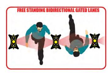
Since this configuration does not require any tethering, units may be powered on at any time and do not need to be facing in any particular direction. Press the POWER button on the first unit and wait a few seconds for the VOLUME button to blink. Next, turn on the second unit and wait for that ALERT button to blink. Continue doing this to as many units as you would like to align for a full gated effect.
