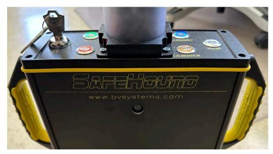
SafeHound buttons are color-coded to match the color of the LED alerts and configuration modes in the pole. Some buttons are multi-function and may require holding down in combinations during specific function states to unock different detection configurations. This user manual corresponds to controller version 1.0.12 Consult this manual fully and included quick start guide for more details.
