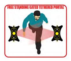
Setting up this configuration is simple. Be sure both units are placed a few feet apart (you can adjust final spacing later) and that the IR sensors are facing each other. The alert LEDs on one side of the poles, the buttons and the SafeHound etching on the base should all be viewable and easily accessible from the outside of the portal allowing only foot traffic within the portal to be detected as they pass through.
