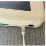
WatchHound-Pro can be updated via its USB-C port connected directly to a Windows PC. The USB-C port also allows the unit to be connect to a PC for live data logging and monitoring. Contact your BVS sales or support representative for more information on the optional PC software.
