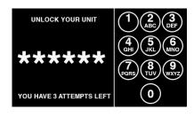
WatchHound-Pro's touch screen requires a six digit PIN code in order to make any changes using the touchscreen even while the unit is physically unlocked. The PIN code is preset at the factory. If you lose your PIN code, contact BVS at 732-548-3737 or support@bvsystems.com.
