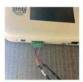
WatchHound-Pro includes dry contacts allowing users to connect external alarms and recording devices upon wireless detection. Contact your BVS sales or support representative for a complete list of supported devices that can be triggered by the dry contacts.
