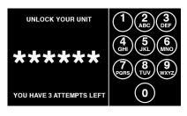
WatchHound-Pro's touch screen requires a six digit PIN code in order to make any changes using the touchscreen even while the unit is physically unlocked. The PIN code is preset at the factory. If you lose your PIN code, contact BVS at 732-548-3737 or support@bvsystems.com.
