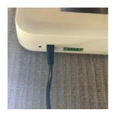
WatchHound-Pro can be powered in 2 different ways. The included 12VDC power allows the unit to operate anywhere. The ethernet PoE (Power over Ethernet) port allows the unit toi be powered over a network connection providing that the cable used is CAT5 or higher capacity.
