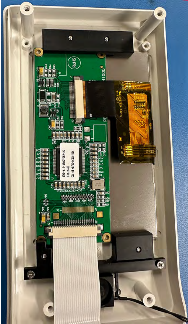
BlueSleuth-Pro Touchscreen, Controller Board & Speaker
