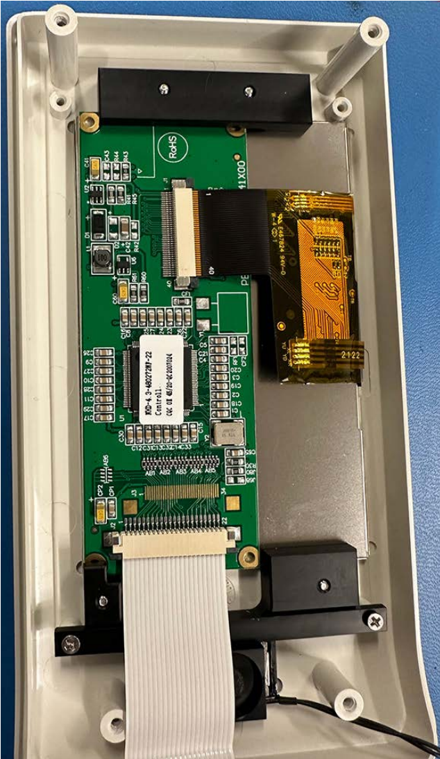
BlueSleuth-Pro Touchscreen, Controller Board & Speaker
