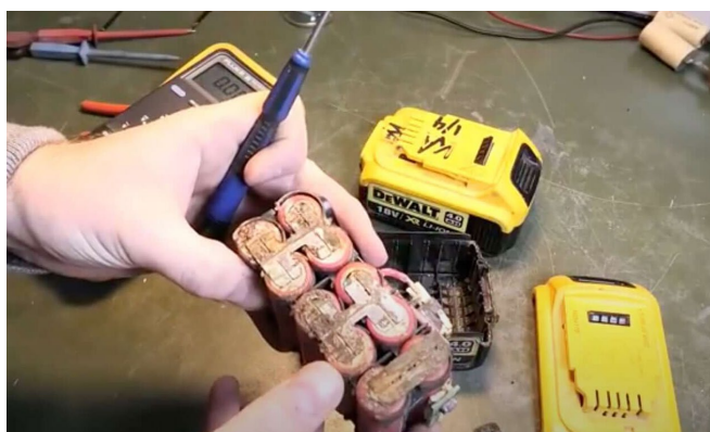
DeWalt XR 18650 4.0Ah battery pack teardown.
