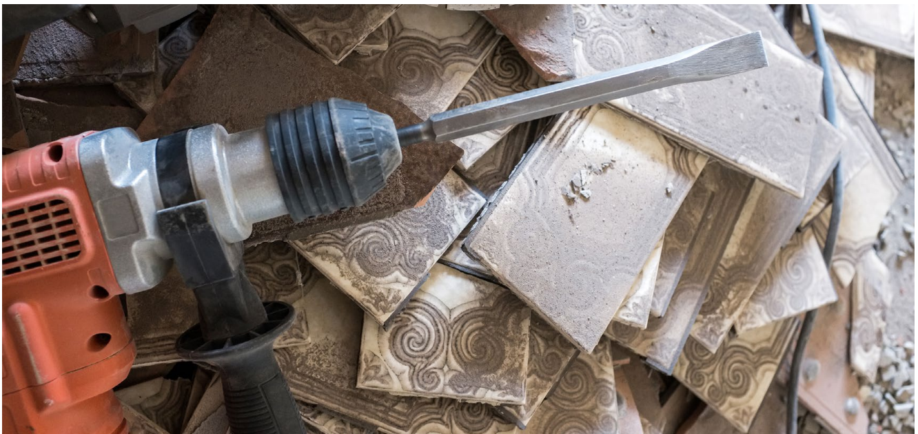
A good rotary hammer can make a tough demo job removing old tiles both quicker and easier. Cordless versions have become lighter and more powerful.
