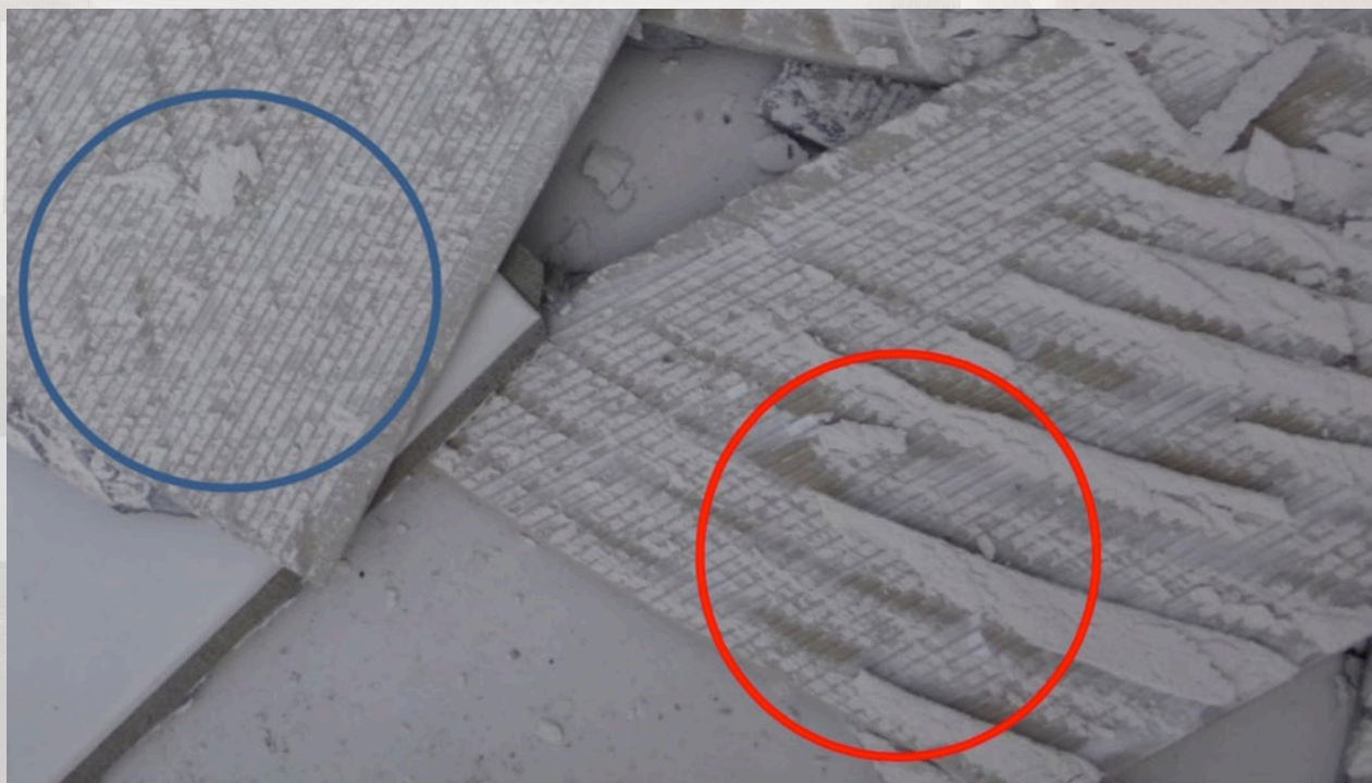
FIGURE 4. Cohesive failure of the adhesive is a common factor (some adhesive left on the substrate, and some on the tile, indicating a shearing of the adhesive itself from excessive stress). Here there are areas of close to 100% adhesive coverage (blue circle) and areas where a “mixed mode” of failure is present (red circle). Sometimes the shearing was perpendicular to the notched adhesive and a regular peaked or wave like fracture was observed. (See Figures 5 and 6)
