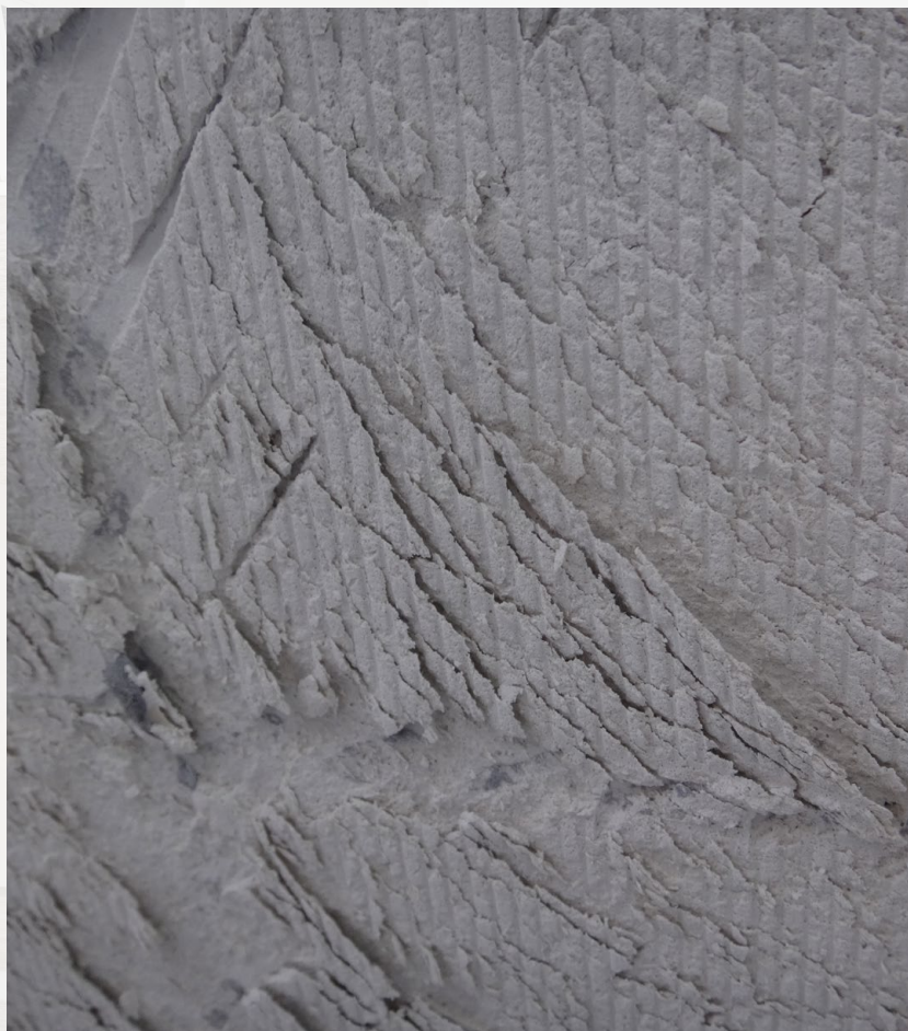
FIGURE 3. Delamination still occurred when 100% adhesive coverage was present. The directional rills in the adhesive indicate the direction of the shear stress.
