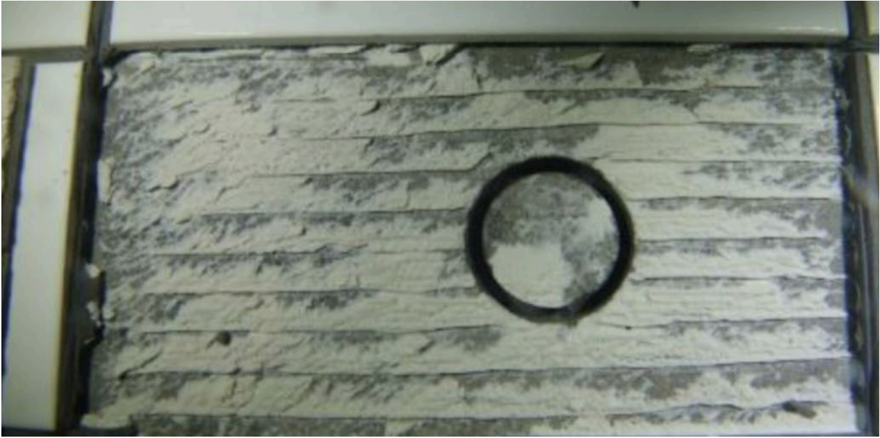
FIGURE 5. The shearing pattern looks similar to waves breaking on a beach.
