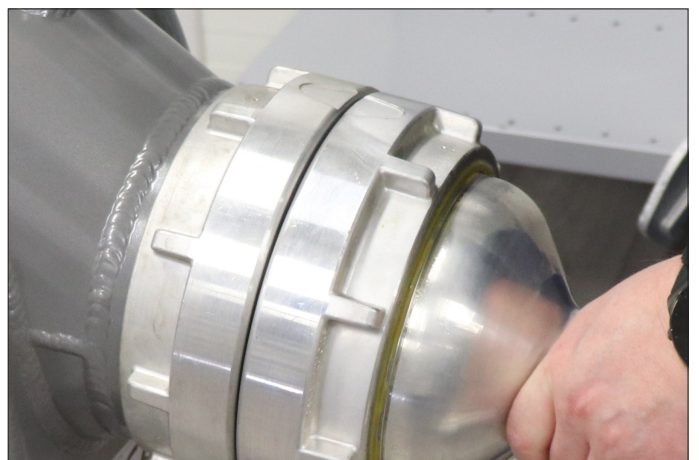
3. The Storz nozzle is locked when the connecting symbols are aligned.
