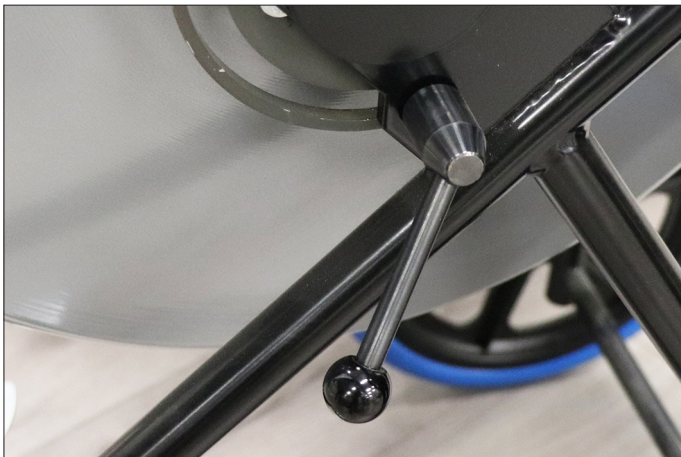
10. You can adjust the drum installation angle by loosening the lever, then turn the angle to fit and tighten.
