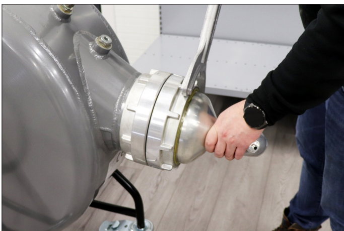
2. Lock the Storz nozzle on the drum by turning it with the Storz key.
