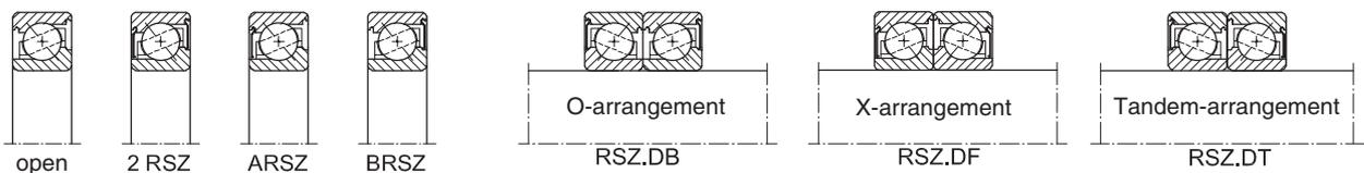
Open, sealed 40° angular contact ball bearings as single and matched bearing sets
