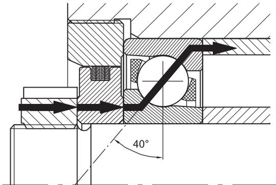
Load acting of 40° angular contact ball bearing
