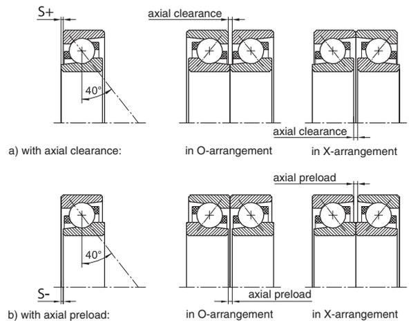
Bearing arrangements with axial clearance and axial preload
