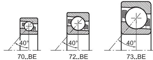
Comparison of cross sections of 40° Angular Contact Ball Bearings 44-102
