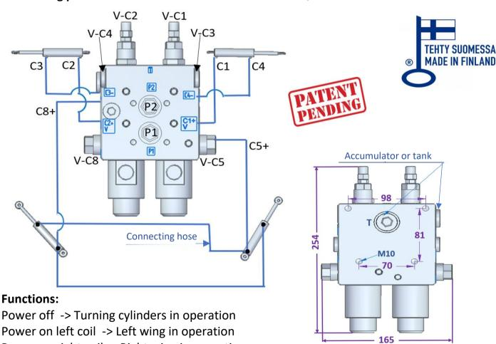
Power on left coil -> Left wing in operation Power on right coil -> Right wing in operation Power on both coils -> Wings simultaneously in or out (wings connected in parallel without flow distribution)
