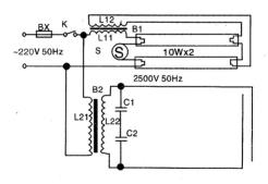
B1-lamp ballast B2-high pressure transformer K-switch S-lamp starter BX-power fuse C-capacitor
