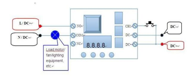
**Gentle remind:** If user load and FRM01 module use a seam DC power supply, it is possible because of the power supply capacity is insufficient or wiring connections unfit, the module appears unstable phenomenon occasionally, please use the following (even if no found the problem, it should follow the recommendations):
