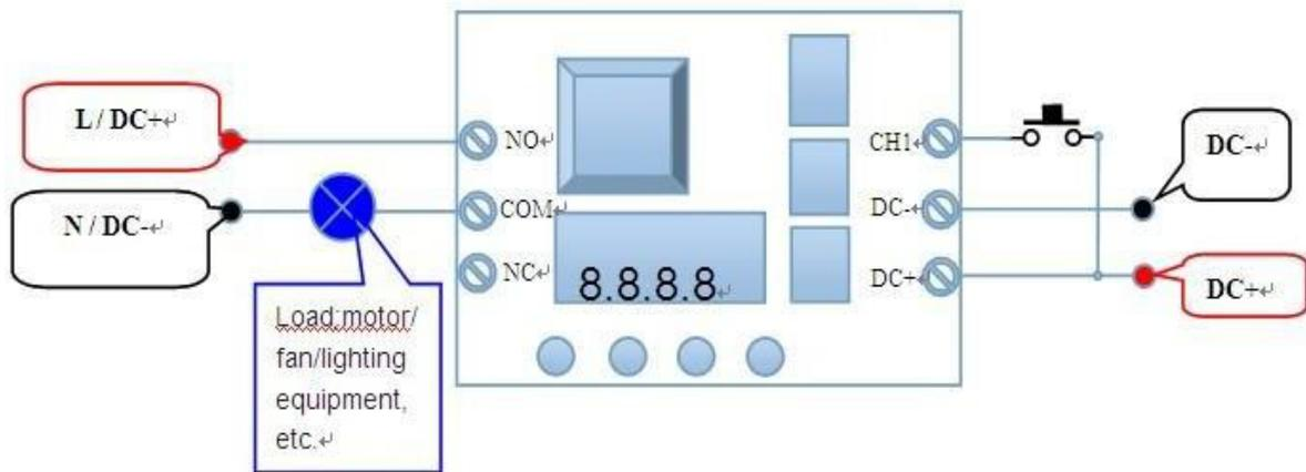
**Gentle remind:** If user load and FRM01 module use a same DC power supply, it is possible because of the power supply capacity is insufficient or wiring connections unfit, the module appears unstable phenomenon occasionally, please use the following (even if no found the problem, it should follow the recommendations):
