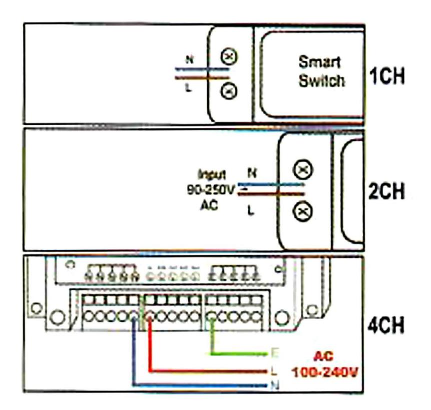
4.1 N+L 2-Wire connection: (Earth wire is not essential for 4CH, example: lamp/fan)
