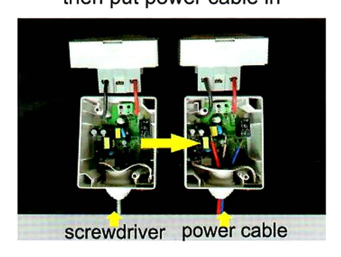
Connect the wire to the appropriate location It will be locked When you put the N and L in the hole Use a screwdriver to press it down when you pull it out
