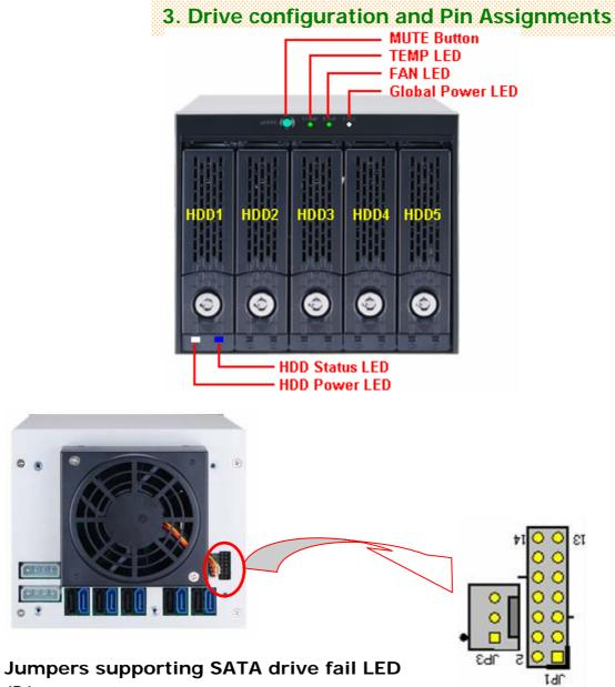
JP1 Pin 1,3,5,7,and 9 – GND Pin 2,4,6,8 and 10 – HDD Fail LED input (Active Low)
