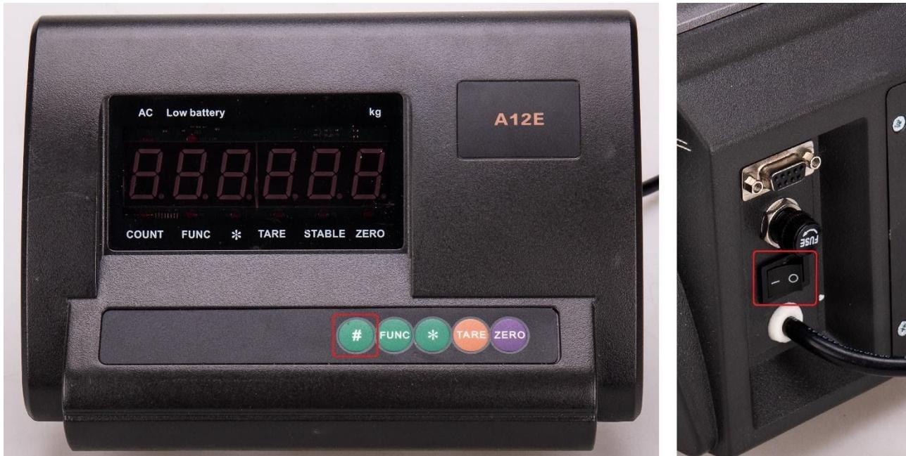
We will stop pressing the "#" key when the number 9999 appears on the screen and it stays on that screen for 2 seconds. Then we release and this screen will appear. We will leave it as it appears in the photo:
