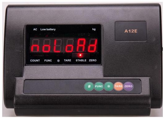
In this case, DO NOT PLACE weight on the scale. With the scale without weight and the STABLE LED on, confirm with "#" and jump to the next screen:
