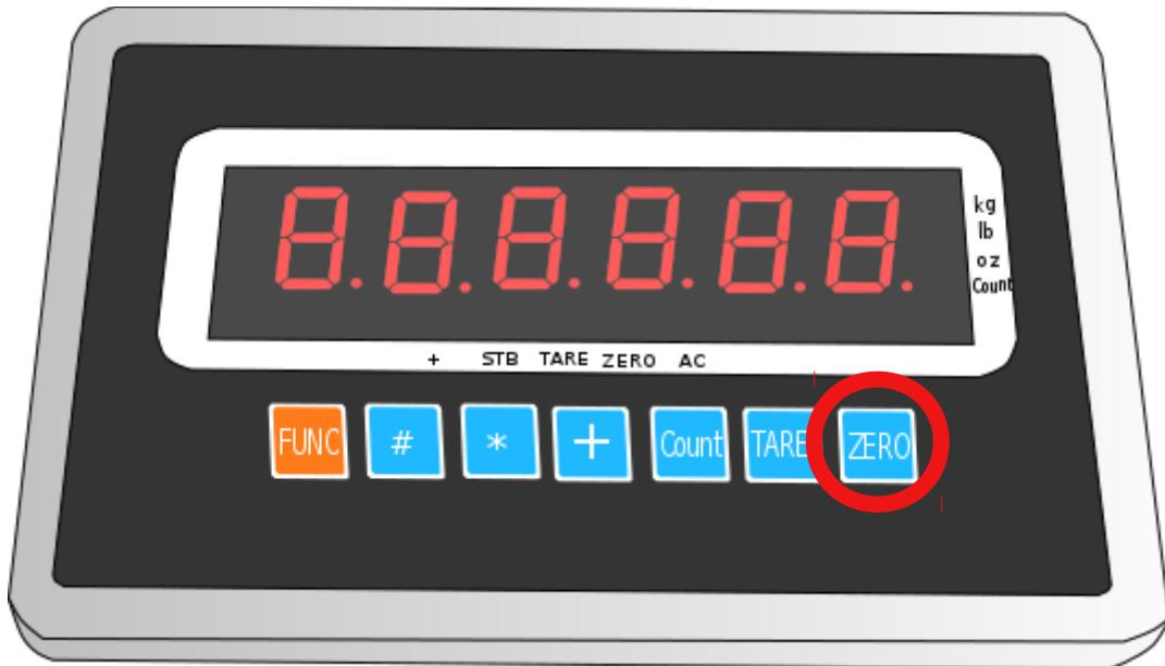
With the ZERO key pressed we turn on the scale.
