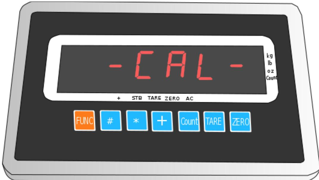
At this point we must enter the weight that we are going to place on the scale, that way the scale will have a weight reference.
