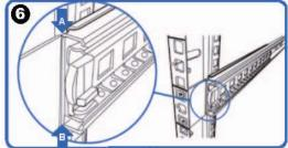
Align front outer rail to the indent of L bracket between Point A & B.
