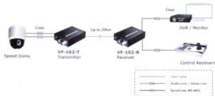
Figure 3-1 VF-102-T / VF-102-R stand alone installation
