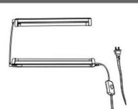
Connection method as shown: use double-ended line to connect the two lamps.
