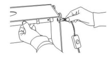
Take out power cable. Insert shape "8" plug from left or right into oval hole on side board. You can loosen the knob a little if the screw prevents you doing.
