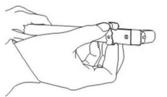
Clip the hook of light tube on the light tube base, one on each side.
