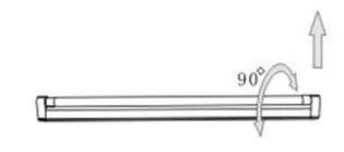
Turn off power when changing light tube. Swivel light tube 90° upward and take out light tube.
