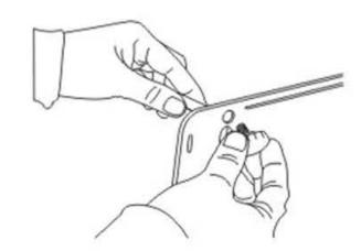
Fix aluminum alloy tube and sideboard together with screw
