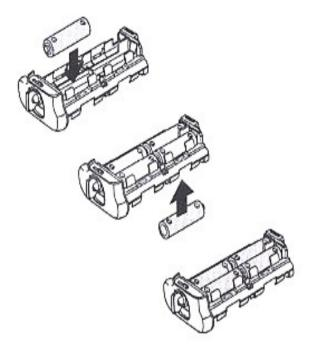
4. For AA batteries: Place sixAA batteries of the same type in the AA battery holder, while ensuring that they are in the correct orientation . Mixing the old and new batteries may cause accident.
