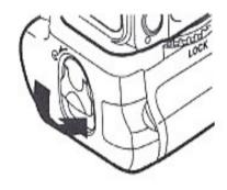
5. Insert the battery holder into the grip. Close the battery chamber and then turn the latch clockwise to lock. Turn on the camera and switch the control lock to be on "." position, and then check the battery level in the control panel or viewfinder.
