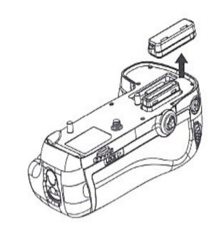
Remove the contact cap from the BG-2N battery grip.
