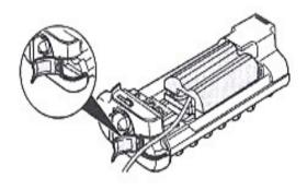
6. To use the EP-BS DC coupler (sold separately), insert the adapter into the EN-EL15 battery holder in the same manner as a regular battery.
