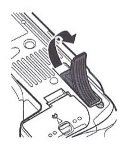
The contacts for the BG-2N are on the bottom of the camera where they are protected by a contact cover .Remove the contacts cover before mounting the grip.
