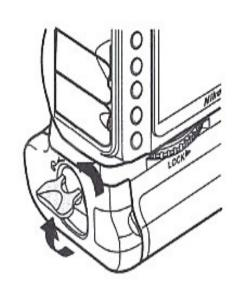
Ensure that the power is turned off on the camera and the control lock on the BG-2N is in the "L" position .Turn the battery-chamber latch counterclockwise to open the battery chamber door.
