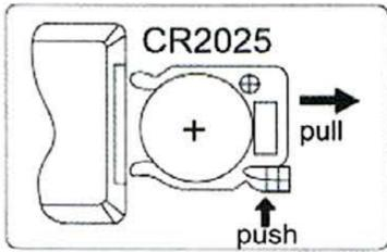
1. The battery compartment is located on the narrow side of the remote control. Pull it out as shown.
