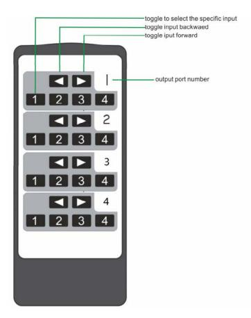
User can control the HDMI route of the matrix by using the IR remote. There are four group key pads for four output ports. For each output port source selection, there are 4 number keys and two arrow keys. Press number keys to select specific input port. Left arrow button to backward the input port, and right arrow to forward input port.
