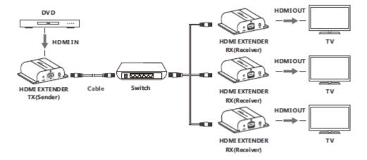
Note: Gigabit (1000Mbps) switcher is Recommended in LAN transmission.
