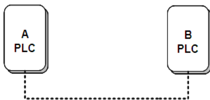
Figure 16 Forming a HomePlug AV logical network
