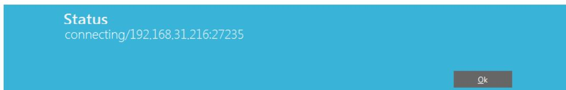
When this USB serial device is connected by other users on the network (Internet/LAN/WAN), it will show “connected/192.168.31.8:27251 (IP address and TCP port number of remote shared USB device)/TITAN-TEST-PC (client computer name or IP address)”.
