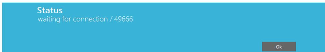
When this USB serial device is connected by other users on the network (Internet/LAN/WAN), it will show “connected/xxxxx (TCP port number)/john-PC (client PC name or IP address)”.
