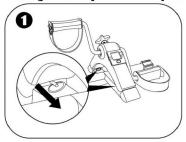
Pull firmly on the ring at the joint of the frame leg.
