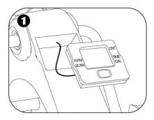
Remove the screen unit from its socket.
