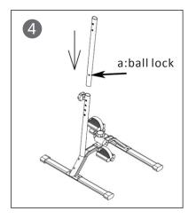
4. Press the ball lock and insert the upper main stem into the lower part until the ball lock stuck into the hole.
