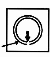
3.Insert the ventilator into the glass hole according to the drawing, rotate the main body to the normal position, and inject the surrounding area with the glass glue to tighten it
