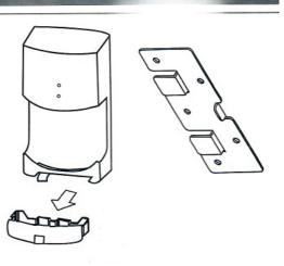
2.hand The Main Body Into Metal Installation Board .( Pic As Below)
