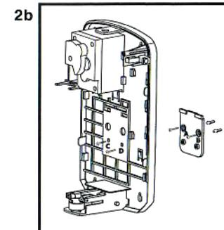
Remove the chamber, Using bracket as guide, mark and drill 2 center holes(AB). Insert anchors into holes, screw fasteners halfway into anchors. Mount bracket onto fasteners and tighten fasteners. Hang the dispenser on bracket firmly. Screw fasteners into installation holes(CD) in backplate and through bracket. Be careful not to over-tighten
