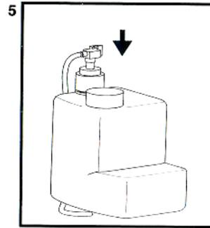
Remove cartridge from dispenser. Remove lid from cartridge. Fill with liquid soap/alcohol and replace cover. Put cartridge back into dispenser. Priming the dispenser will take six to ten pumps.
