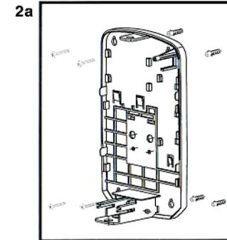
Using backplate as template. Mark the location for 4 mounting anchors. Drill holes and insert anchors into holes, screw fasteners halfway into anchors. Mount dispenser onto fasteners. Tighten fasteners (Do not over tighten).
