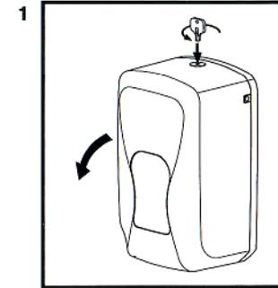
Use provide key to open the front cover. Insert the key into the holes located at the top of the dispenser, twisting the key, and pulling the cover towards you. The cover is hinged at the bottom of the dispenser.
