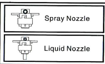
Loose clamp and replace the nozzle. Clip the clamp back to the original position. Make sure that the nozzle of the pump is fixed into the groove.
