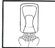
To activate dispenser, place hand under bottom of dispenser. If a second dose is needed, remove hand, and then replace hand under dispenser (when an object comes within 4 inches of the sensing window the dispenser will activate)
