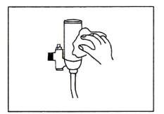
After installation, please use a softcloth to clean the reaction window, make sure the reaction window is clean.
