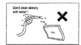
In daily usage and guarantee, the machine appearance should be cleaned with clean and safe cloth instead of cleaning it with corrosive detergent and water, or its appearance and wire inside will be demolished.
