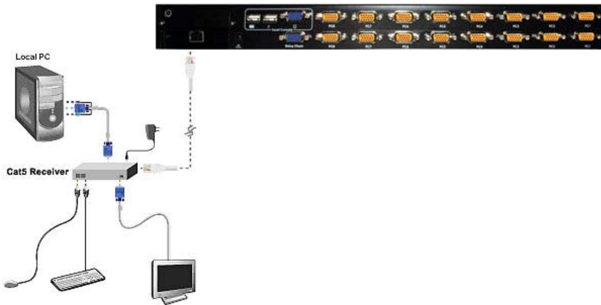
Figure 14. Connect to CAT. 5 Receiver (R-Box)
