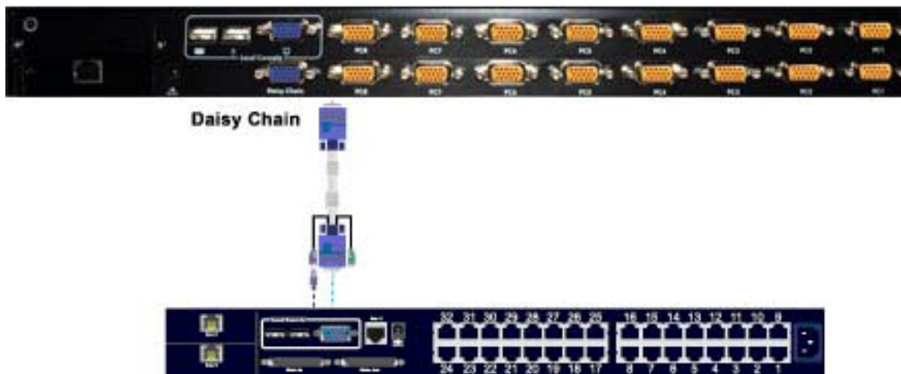
Figure 16. Daisy Chain through Computer Port
