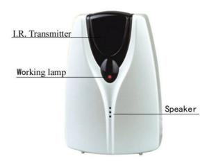
**Infrared Transmitter**: Emits I.R.codes to control the air conditioner's working status.
