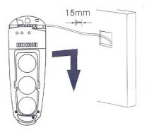
5.Connect the cable to the wire terminal.
