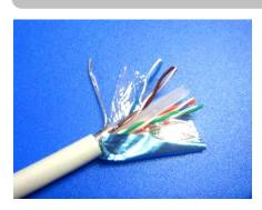
Jyh Eng Category 6 FTP cables are designed to meet the most advanced FTP cable applications. Tested to 250 MHz, the guaranteed performance of this cable meets the ISO/IEC 11801 and EN50288 requirements for PS-NEXT, attenuation, return loss, attenuation-to-crosstalk ratio (ACR) and impedance, making it ideal for high-end transmission links supporting today's networking protocols
