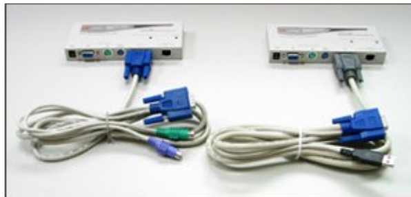
Cable type: 3-in-1 cable for PS/2 computer, CC51 (left) 2-in-1 cable for USB computer, CC56 (right)
