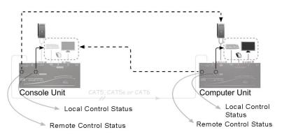
The LEDs on the KVM Extender show the latest status which indicates the linking, communication, and control situation between the Computer Unit and Console Unit.
