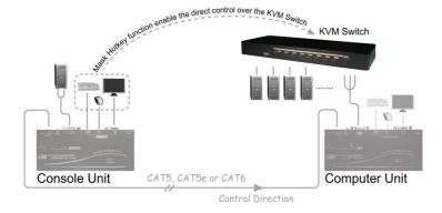
A Mask Hotkey Switch located on the rear panel of both Console Unit and Computer Unit can be slid ON/OFF to switch hotkey control between the KVM Switch cascaded / Computer connected accordingly. Through sliding Mask Hotkey Switch "ON" to mask up the Extender Unit itself, as if users actually sit in front of the KVM Switch to directly configure the attached computers by applying the KVM Switch built-in hotkey commands.
