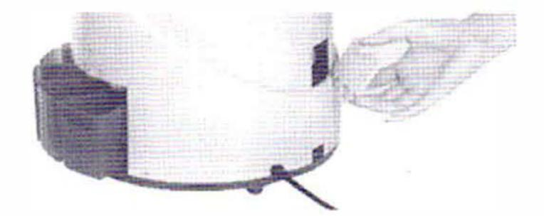
2.To remove any trapped coin, follow picture shown below, use a finger to push up the jammed coin and let it fall out from the gap between the channels.
