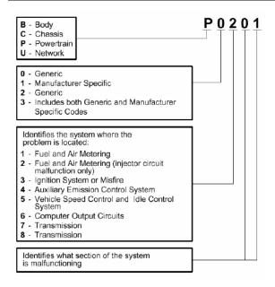
P0201 - Injector Circuit Malfunction, Cylinder 1
