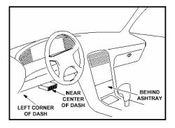
The 16-pin DLC is usually located under the instrument panel (dash), within 12 inches (300 mm) of center of the panel, on the driver's side of most vehicles. It should be easily accessible
