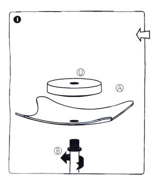
Insert assembled tube (B) into base (A) and screw on holder.
