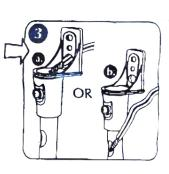
FOR LOUDSPEAKERS WITH THREADED HOLE Secure universal bracket(h)to upright using screw(i). The speaker cable should be Connected to the speaker and threaded through the upright as shown in fig 3a or 3b. The speaker should be fixed to bracket (h) Using washer(r)and either screw(o) or (p) depending on speaker type, Fit cover cap (k) if required.
