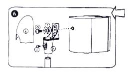
BOSE ACOUSTIMASS LOUDS PEAKERS Attach universal bracket(h) to pole using screw (i) Feed cable down pole as shown in fig 3a or 3b. Attach loudspeaker to bracKet using screw (o) and washers (r).
