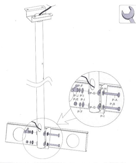
Assemble the universal plate and bottom pipe with connect plate. Using correct combination of screws, washers, nuts and iron knob.
