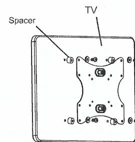
Install mounting panel to bent back of TV
